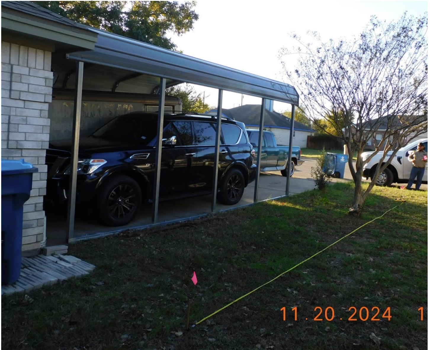
Photo #4 shows measurement #1 from the slab to the side property line (7.0') and measurement #2 from the side property line as indicated by the pink flag in the photo above toward the street (25.5') for the approximate front property line.
